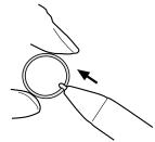
To remove the old nib: Clasp it with a pair of tweezers, needle-nosed plier, or similar instrument and pull the old nib straight out of the pen.
